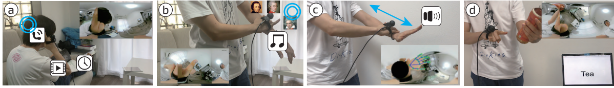
Figure 6: (a) Location detection can trigger corresponding apps. (b) The combination of hand location and posture can realize information storage in a hierarchical manner. (c) Hand keypoints detection can enable a stroking action on the forearm to be interpreted as a continuous input. (d) Object recognition can be triggered by pointing at it with the hand wearing the device.
