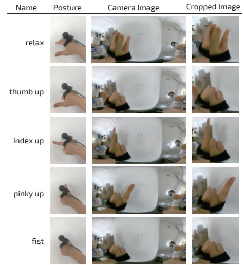
Figure 3: The set of hand postures used with the prototype and the corresponding complete 360^\circ images and cropped images using a predefined ROI.
