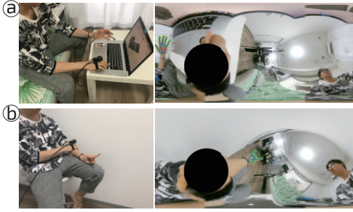
Figure 4: Keypoints estimation of the hand without the device in certain postures. The area surrounding the camera hand is painted black to avoid recognizing the hand with the device. (a) Putting the hands in front. (b) Placing the hand with the device onto the other arm and bending the wrist back.
