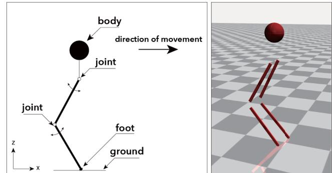
Fig. 3. Robot model used for policy training in the simulation environment.
