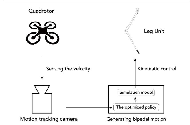
Fig. 6. Control system in the real-world environment.
