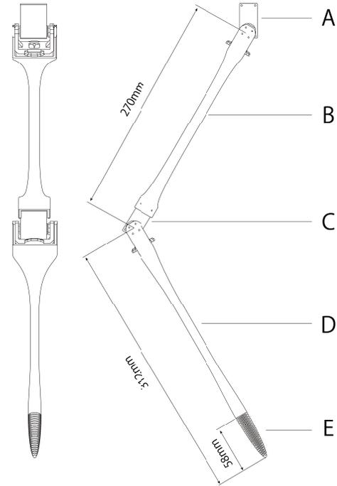
Fig. 2. Components of the leg unit.
