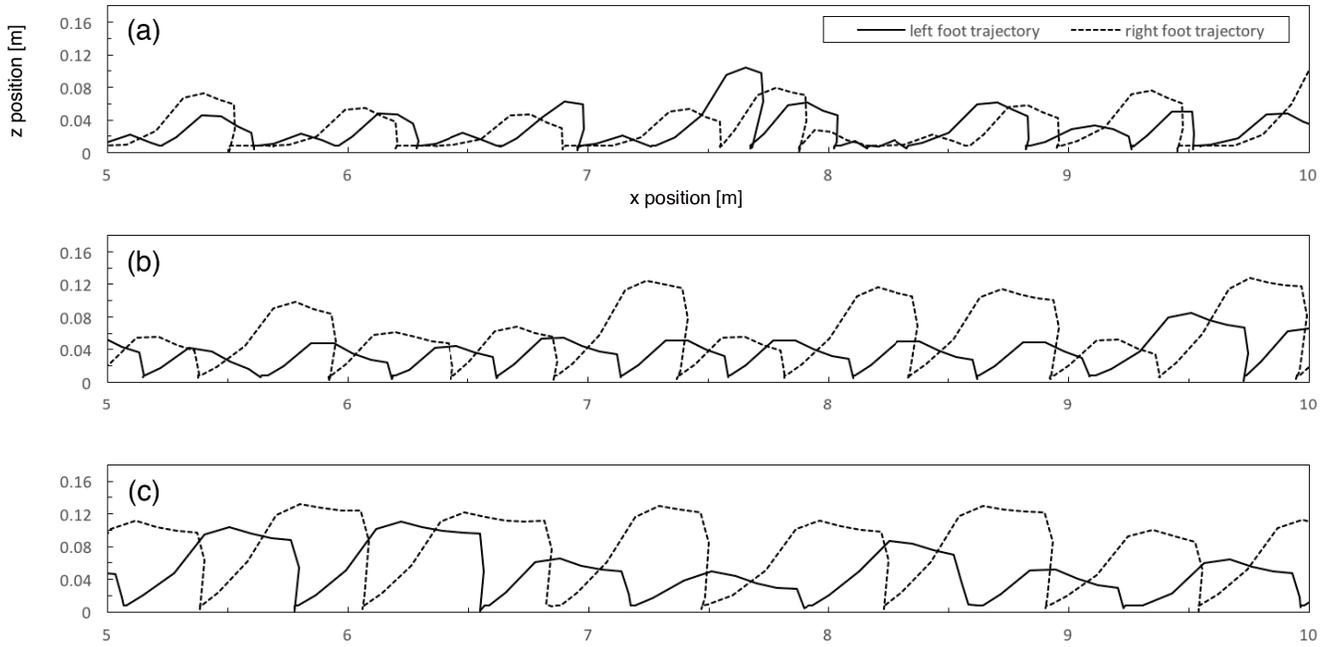
Fig. 5. Foot trajectories at (a)  $v_{body} = 0.5$  m/s, (b)  $v_{body} = 0.75$  m/s, (c)  $v_{body} = 1.0$  m/s ( $5.0 \text{ m} \leq x \leq 10.0 \text{ m}$ )
