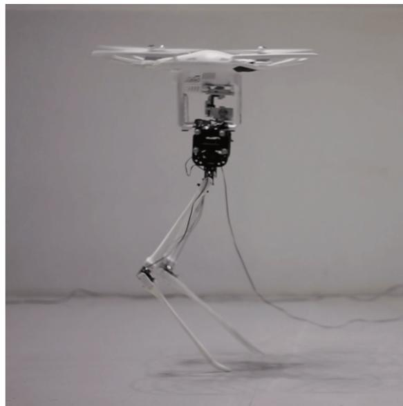
Fig. 1. Appearance of the bipedal robot using a quadrotor.
