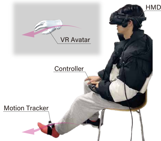
Fig. 1: The redirection detection task conducted in the VR space. Participants used different body parts (their hand and foot), to manipulate a VR avatar and perform reaching movements, with the motion being shifted left or right depending on the experimental condition.
