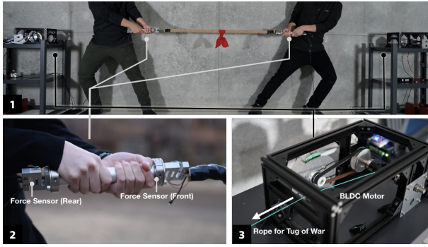
Figure 2: 1) The players pull at the rope using handles. 2) Two force sensors on the handle measure forces at both the front and rear ends, which detects how each player is applying force. 3) A BLDC motor pulls at the rope from behind each player.
