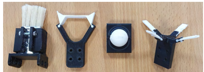
Figure 4: A set of end-effectors: universal fastener, bistable gripper, flexible hemisphere, and 4-legged soft supporter.
